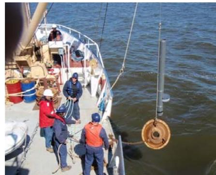
Sequential sediment trap is deployed from the deck of the MV Namao.
